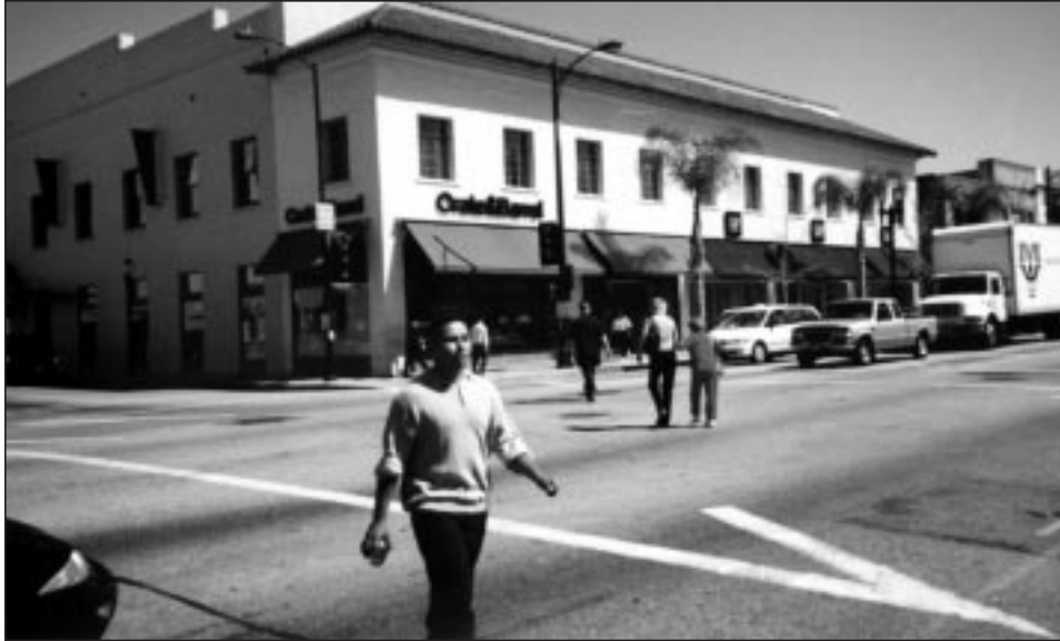
An intersection in which a Pedestrian Scramble is implemented, allowing pedestrians to cross in all directions including on the diagonal.
