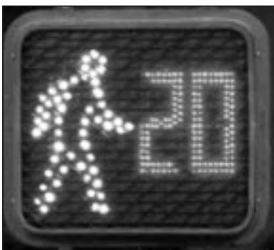
Countdown signals have been added to the Manual on Uniform Traffic Control Devices (MUTCD) as an optional use device.
