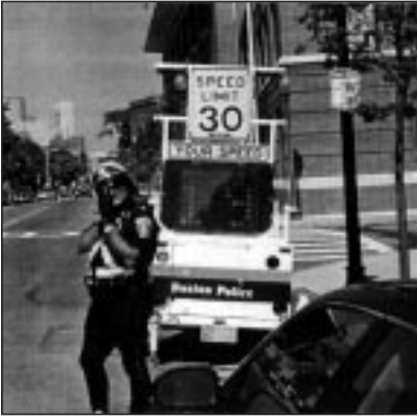
The Boston Police Department uses speed trailers and radar guns to automatically detect and display vehicular travel speeds.
